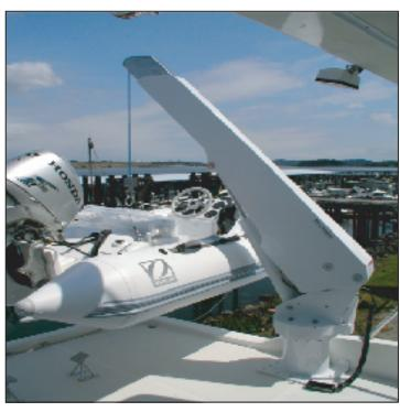
Systems come complete with hydraulic power pack, (choose 12v 24v or 115v.) stainless steel hydraulic hoses, 8 button remote control pendant for 4 Function control and correct paint code to match your specific yacht.
