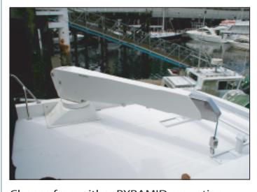
Choose from either PYRAMID mounting, (shown above) or Standpipe Model. (shown right view) We can work with you for your special application as needed.
